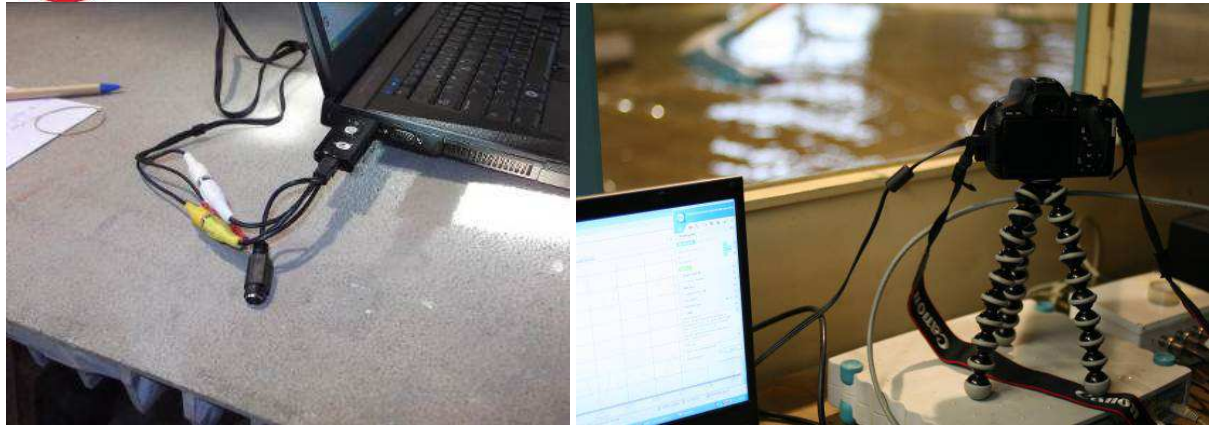
Figure 34 - Cable connections between camera and computer.
