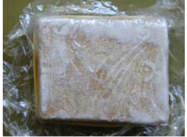
Figure 13. Vapor insulation method A1 of sample A2 using plastic sheet and an elastic. (a) with epoxy resin on the sides; b) With mastic and a plastic sheet after the drying cycle, with massive efflorescence's on the back. .
