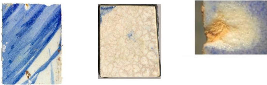
Figure 12. Samples A2 and A5 after 5 and 7 cycles: a) A2 at final cycle Ci5; b) A5 at final cycle Ci7 and c) detail of unglazed area without efflorescence at A2.
