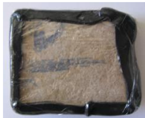
Figure 16. Vapor insulation of sample A2 using Sticky tape AT199 from 3M. (a) with epoxy resin on the sides; b) adding a rigid plastic sheet on the back; c) sealing with Sticky tape AT199; d) Adding a plastic sheet in the end; e) final isolation view from the front; and, f) final isolation view with no efflorescences on the back.
