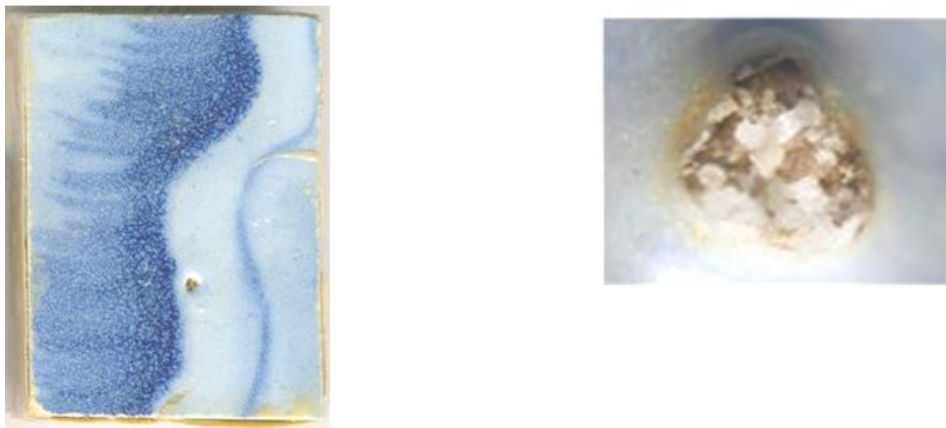
Figure 13. Sample A6a: a) after 8 cycles and b) a detail of the efflorescence's in the glaze pore.
