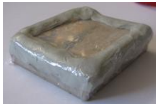
Figure 15. Vapor insulation of sample A2 using Mastic. (a) with epoxy resin on the sides; b) adding a rigid plastic sheet on the back; c) sealing with Mastic; d) Adding a plastic sheet in the end; e) final isolation view from the front; and, f) final isolation view with no efflorescences on the back.
