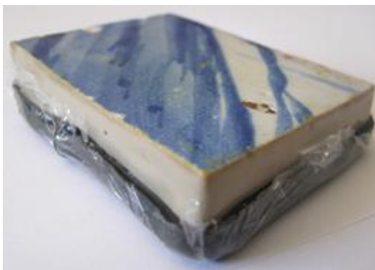
Figure 16. Vapor insulation of sample A2 using Sticky tape AT199 from 3M. (a) with epoxy resin on the sides; b) adding a rigid plastic sheet on the back; c) sealing with Sticky tape AT199; d) Adding a plastic sheet in the end; e) final isolation view from the front; and, f) final isolation view with no efflorescences on the back.
