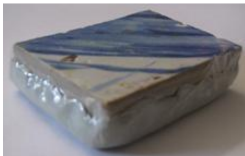
Figure 15. Vapor insulation of sample A2 using Mastic. (a) with epoxy resin on the sides; b) adding a rigid plastic sheet on the back; c) sealing with Mastic; d) Adding a plastic sheet in the end; e) final isolation view from the front; and, f) final isolation view with no efflorescences on the back.
