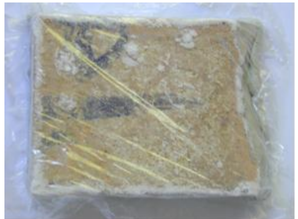
Figure 14. Vapor insulation method A2 of sample A2 using plastic sheet and mastic. (a) with epoxy resin on the sides; b) With mastic and a plastic sheet after the drying cycle, with efflorescences on the back. .
