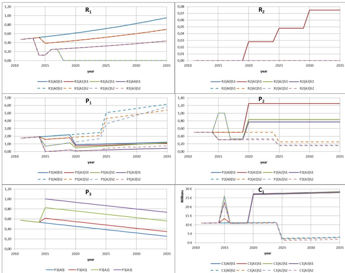
**Figure 3** Time evolution for six assessment criteria: risk of pipe burst ( $R_1$ ); risk of lack of hydraulic capacity of pipes ( $R_2$ ); real water losses ( $P_1$ ); exceeding pipe capacity ( $P_2$ ) infrastructure index value, IVI ( $P_3$ ) and total cost ( $C_1$ )
