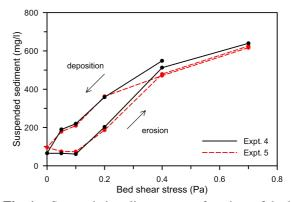
Fig. 1: Suspended sediment as a function of bed shear stress in long-duration experiments.
