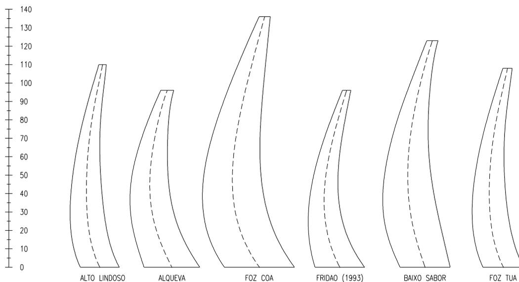
Figure 4: Shape of arch dams crown cantilevers.
