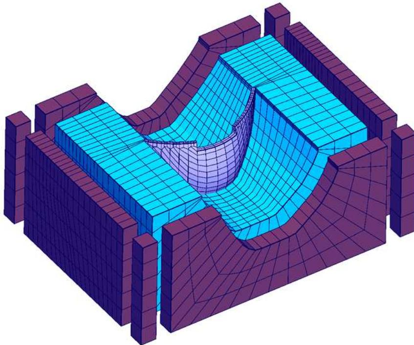
Figure 10: 3DEC model for seismic analysis. Dam with contraction joints and foundation joint, rock mass and lateral free-field meshes.
