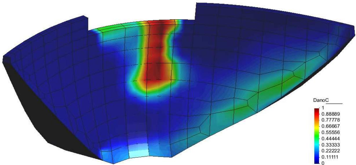
Figure 9: Concrete arch failure model. Contours of compressive damage variable near the structural failure condition.
