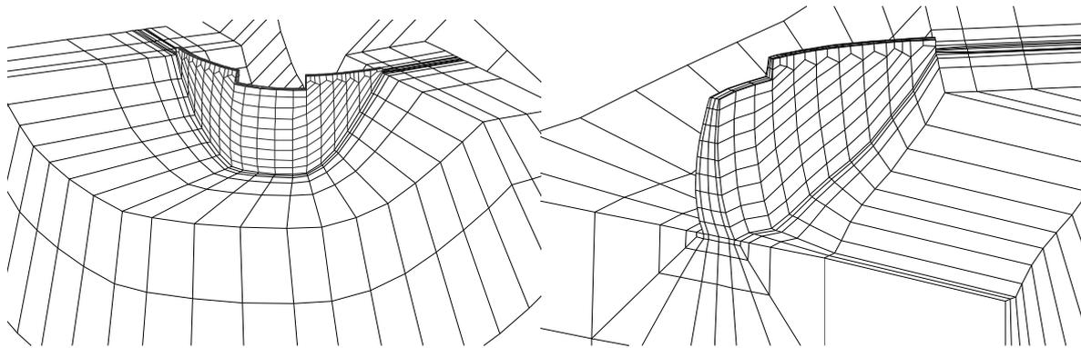
Figure 5: Finite element mesh.
