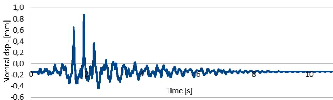
Figure 11: Normal displacement of a contraction joint at the crest (positive is opening).
