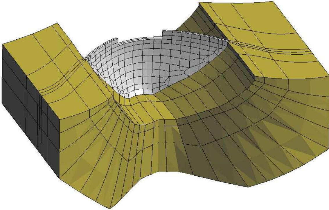
Figure 8: Concrete arch failure model. Finite element mesh.
