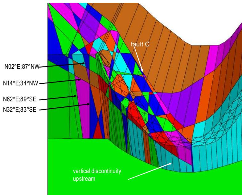
Figure 12: Detail of 3DEC model for the analysis of failure of the left abutment (dam and upstream rock hidden).
