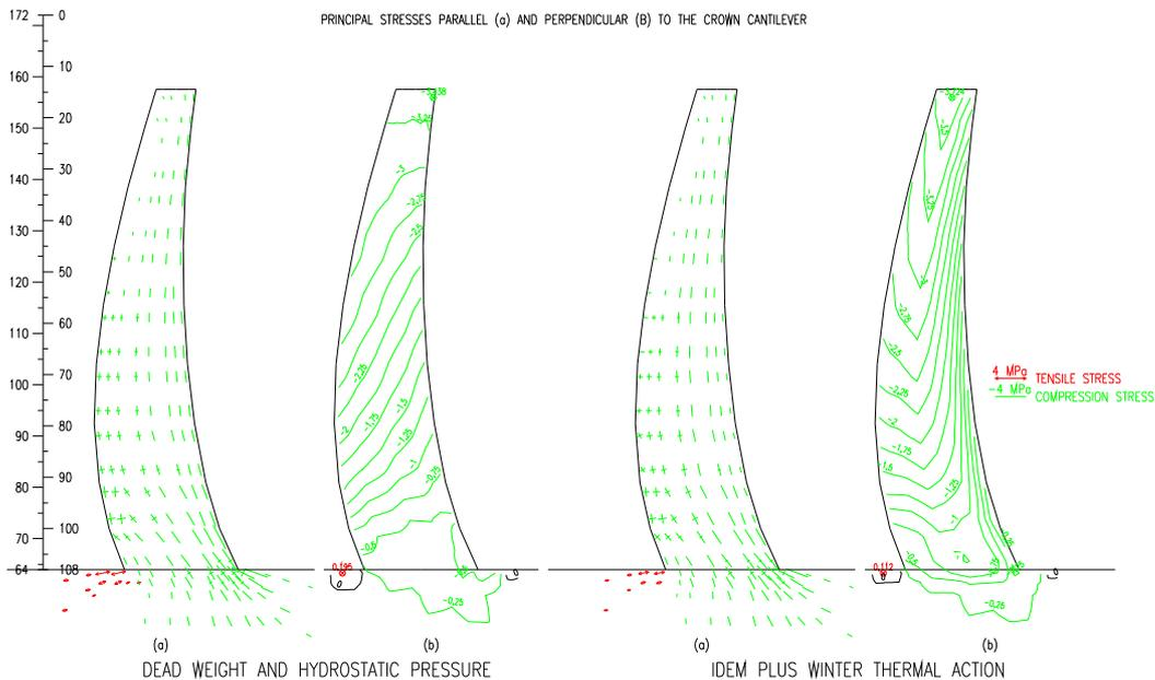
Figure 7: Principal stresses along the crown cantilever.
