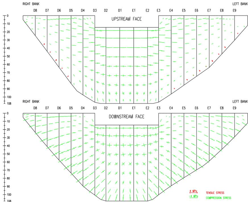
Figure 6: Principal stresses for dead weight and hydrostatic pressure.
