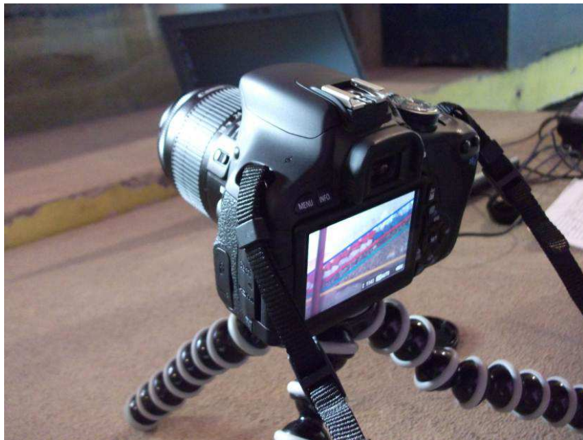
Figure 3 - CO11 flume. Camera held in position using a “Joby GorillaPod® tripod” on a platform in front of the flume.
