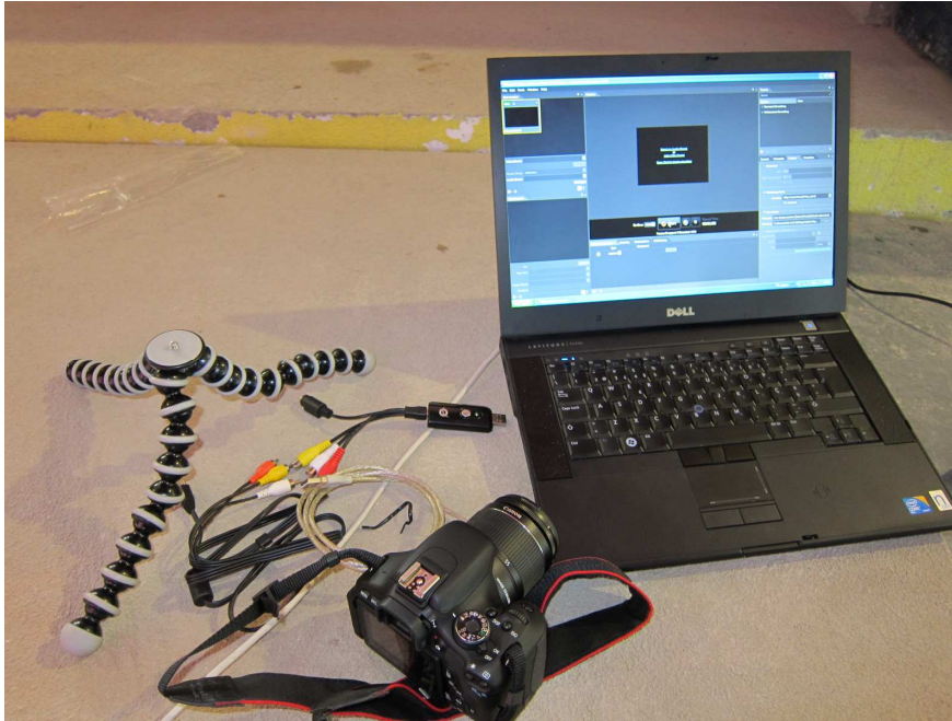
Figure 4 - COI1 flume. Laptop computer (Windows XP, 4 GB RAM) used to both receive conveyed video signal from A/D Converter DAQ board. Also shown are the Canon camera, the Gorilapod, cables (with USB-composite video adapter) and the “USB Conceptronics A/D Converter DAQ board”.
