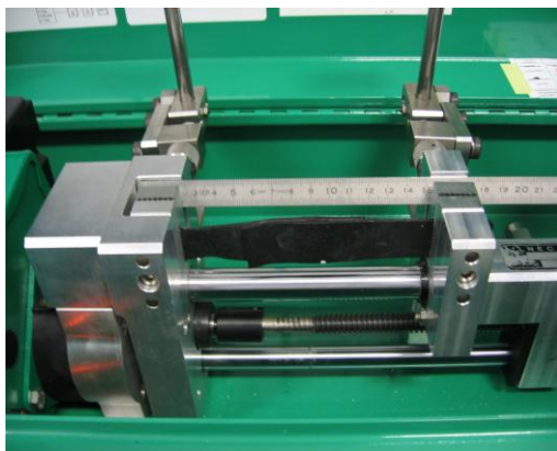
Figure 6. Shear test for seamed geomembranes
