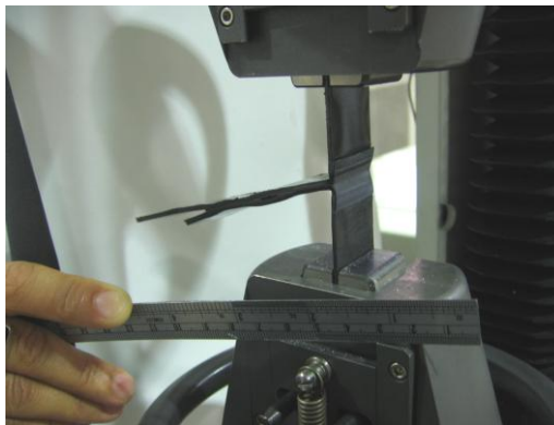
Figure 5. Peel test for seamed geomembranes
