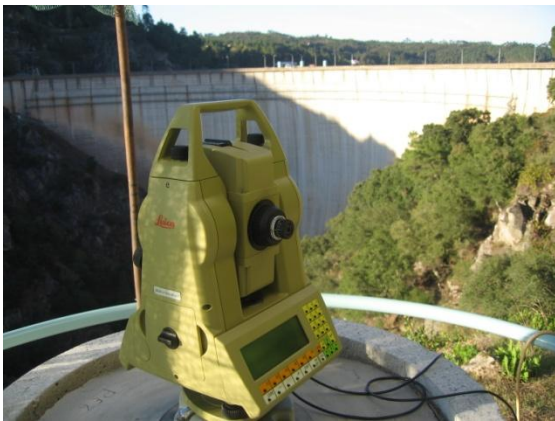
Figure 1 – Tacheometer set on a pillar during the continuous monitoring test
