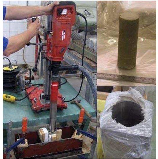
Figure 1. Drilling equipment, sample and prism after drilling.
