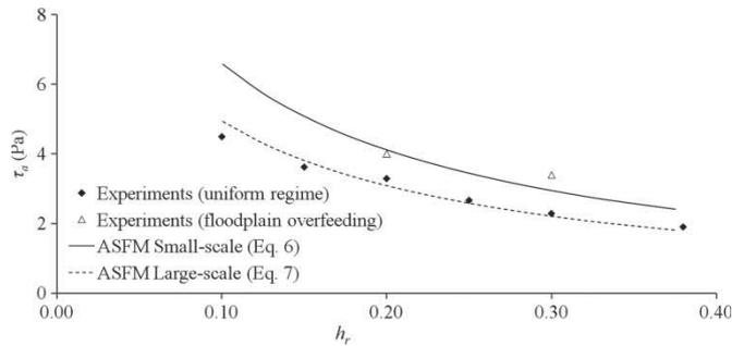
Figure D1 Apparent shear stress versus relative depth for (—), small-scale; (---), large-scale flumes
