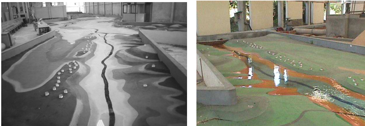
Figure 3: General view of the Arade River valley physical model.
