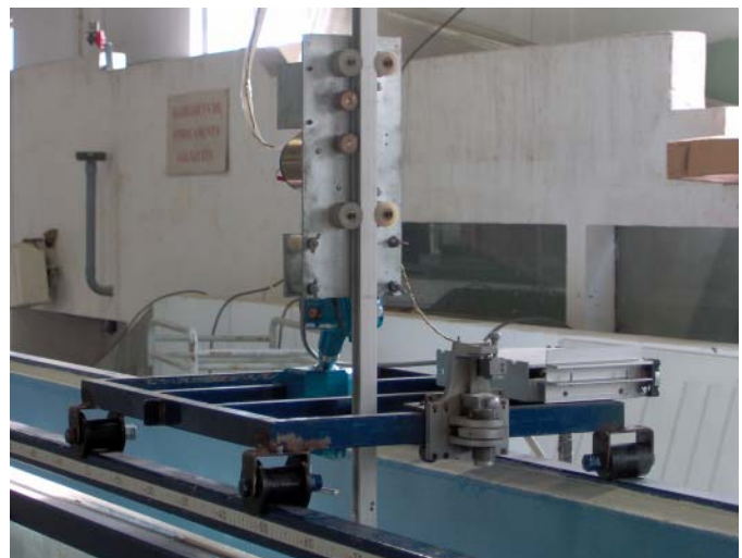
Fig. 8. Photograph showing the external appearance of the instrument block in a flume chariot.
