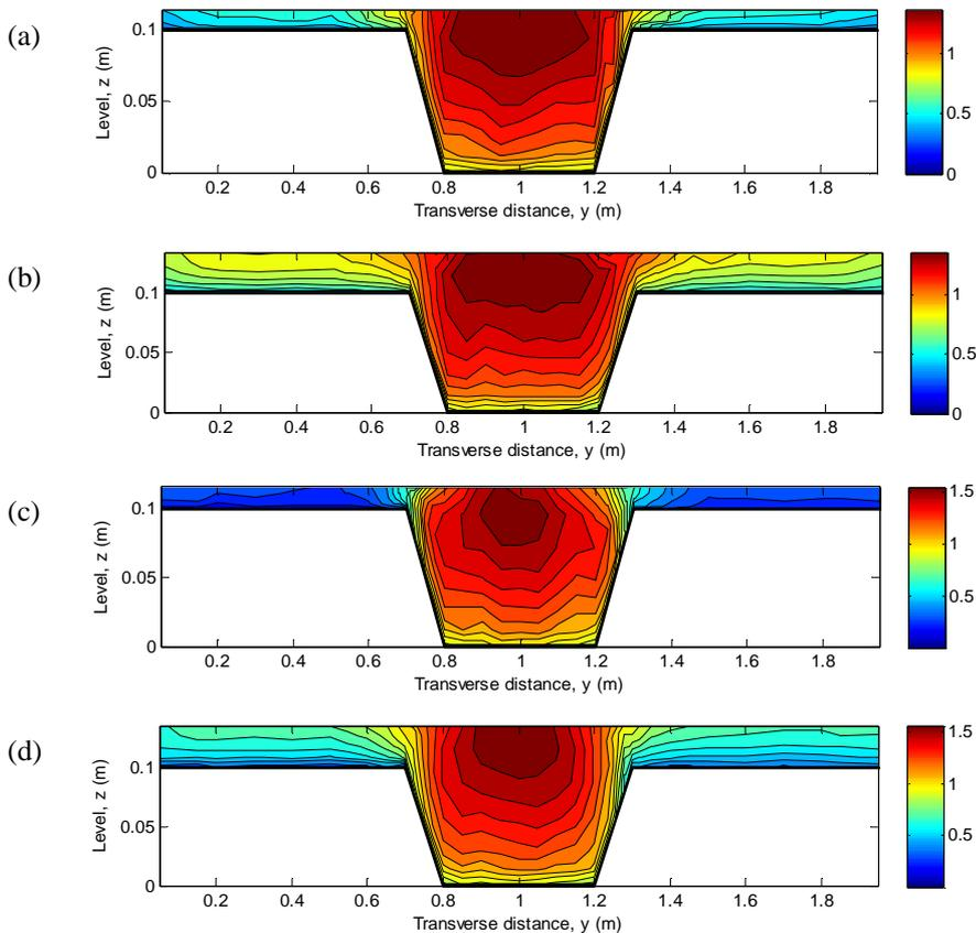
**Figure 4.** Normalized streamwise velocity ( $u/u_m$ ). (a) hr015s; (b) hr03s; (c) hr015r and (d) hr03r
