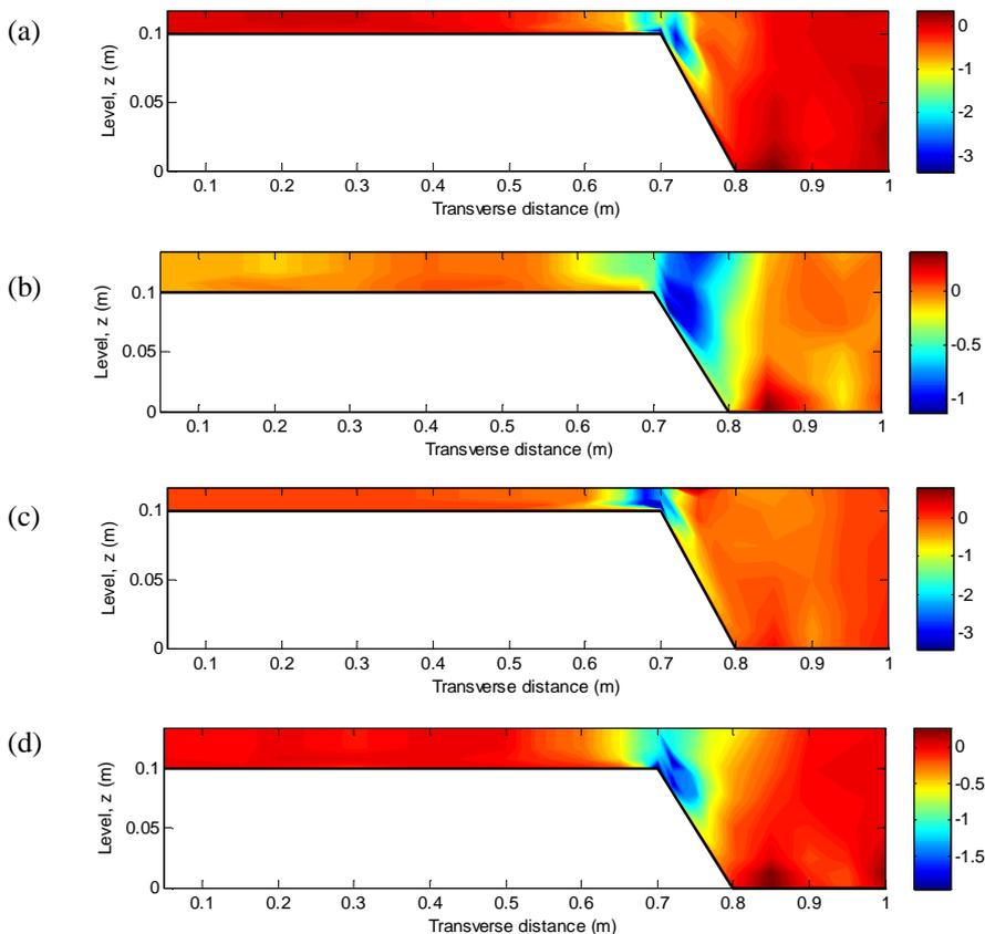
**Figure 5.** Reynolds stresses cross-section distribution ( $\tau_{xy}$  in Pa). (a) hr015s; (b) hr03s; (c) hr015r and (d) hr03r
