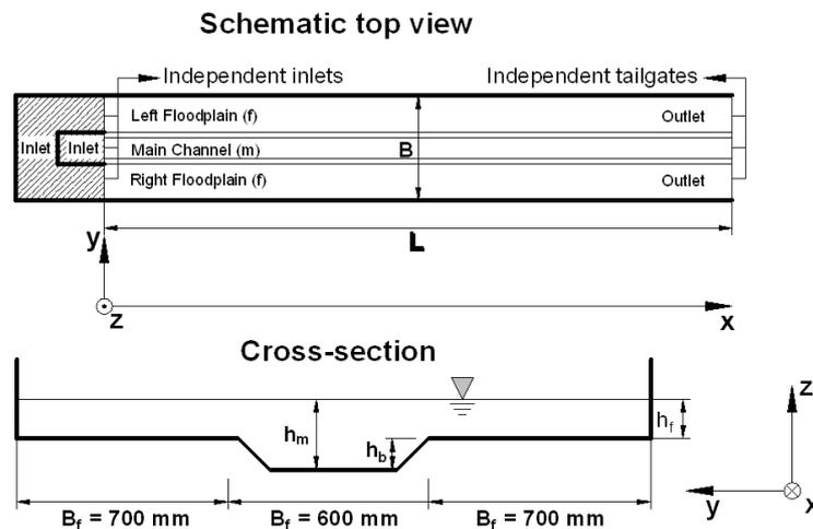
Figure 2. Schematic top view and cross-section.
