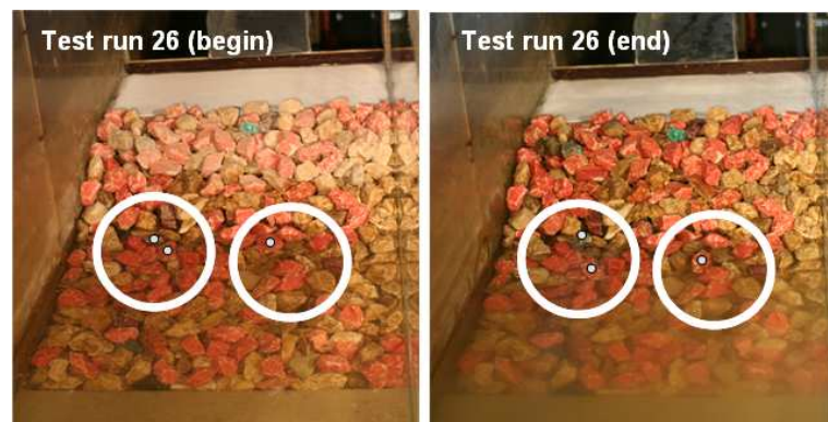
Alternative 3: identification of rock displacements for test run 26 (initial and final rock positions)
