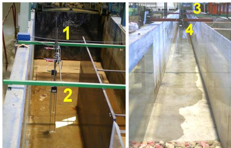
Experimental equipment for free surface elevation: wave gauges
