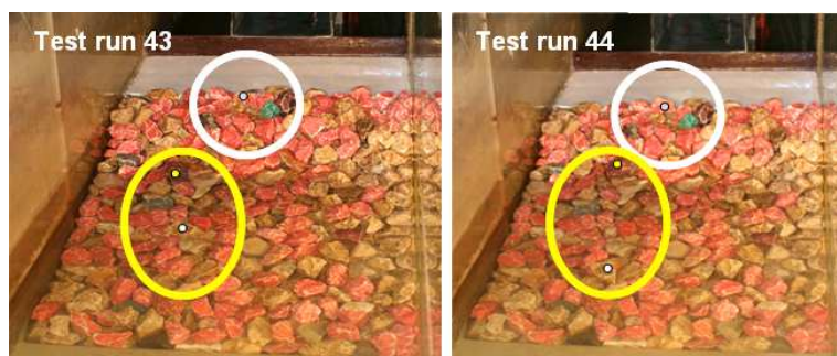
Alternative 4: identification of rock displacements for test run 44 (initial and final rock positions)
