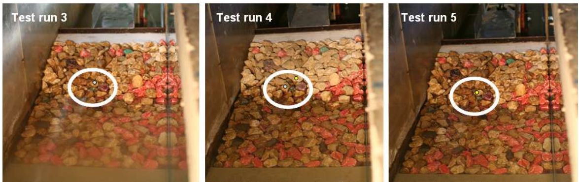
Alternative 1: identification of rock displacements for test runs 4 and 5 (initial and final rock positions)
