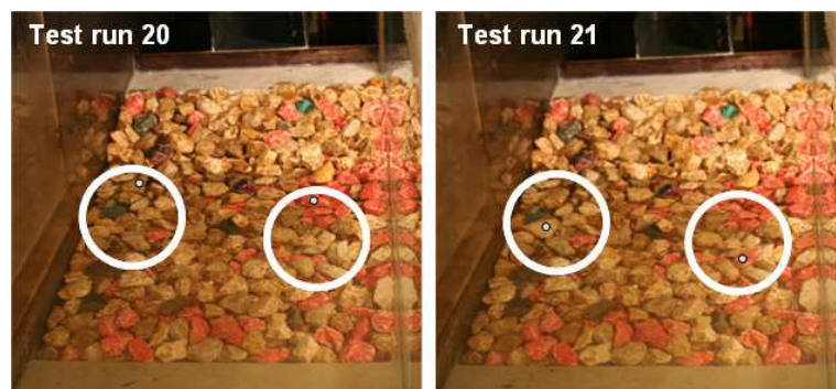
Alternative 2: identification of rock displacements for test run 21 (initial and final rock positions)
