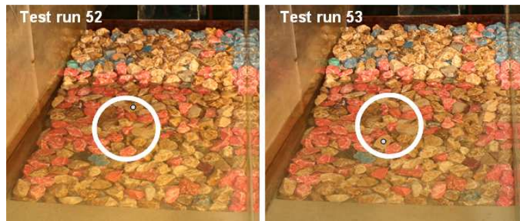
Alternative 5: identification of rock displacements for test run 53 (initial and final rock positions)
