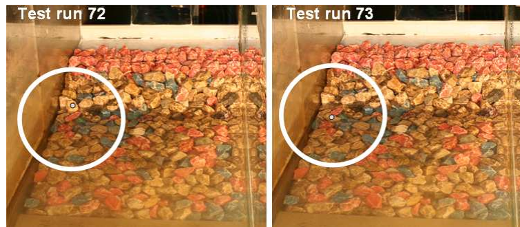
Alternative 8: identification of rock displacements for test run 73 (initial and final rock positions)
