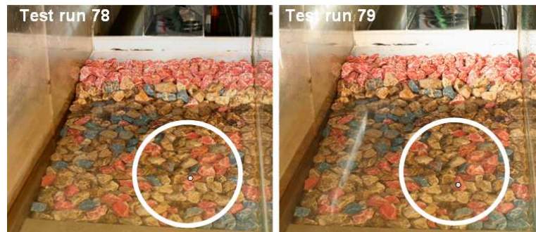
Alternative 8: identification of rock displacements for test run 79 (initial and final rock positions)
