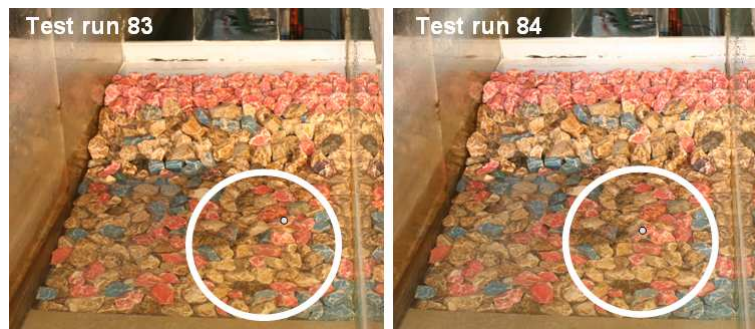
Alternative 8: identification of rock displacements for test run 84 (initial and final rock positions)
