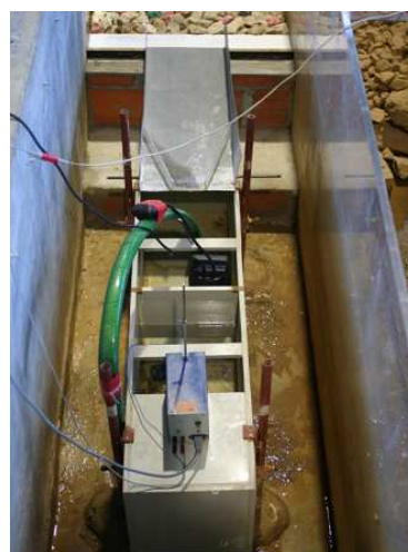
Experimental equipment for overtopping: chute, overtopping tank, water level gauge and pump
