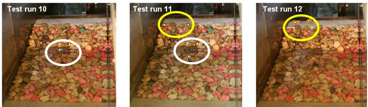
Alternative 1: identification of rock displacements for test runs 11 and 12 (initial and final rock positions)
