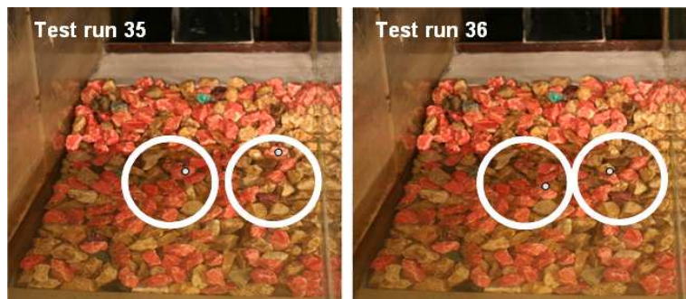
Alternative 3: identification of rock displacements for test run 36 (initial and final rock positions)
