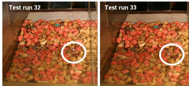
Alternative 3: identification of rock displacements for test run 33 (initial and final rock positions)
