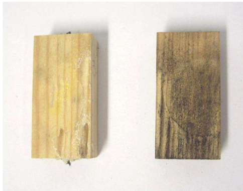
Figure 3: Scots pine sapwood samples after 8 weeks of exposure to subterranean termites, (left) PLEOT protected, (right) unprotected
