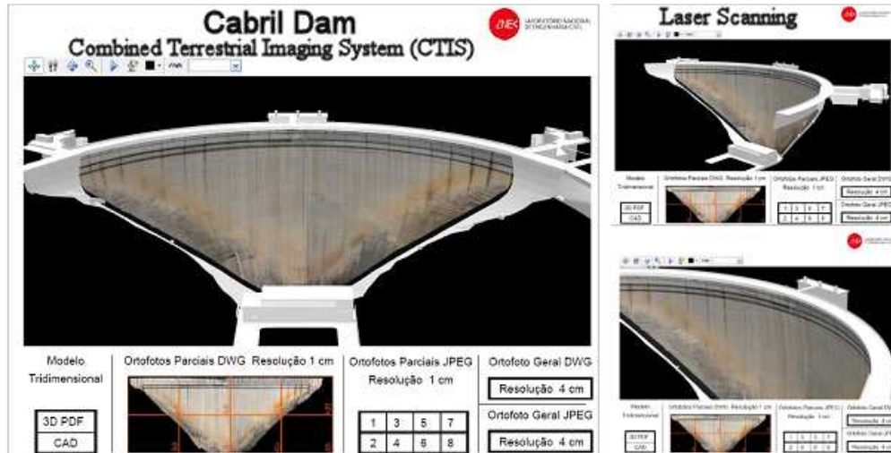
Fig. 8- Several displays of a 3D PDF file with the 3D model of the dam, central image, and links to 1 cm resolution 2D orthoimages [20].
