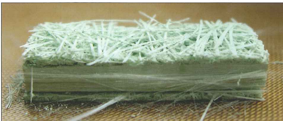
Fig. 2: Outer mats and inner rovings of a burnt laminate (VE profile)
