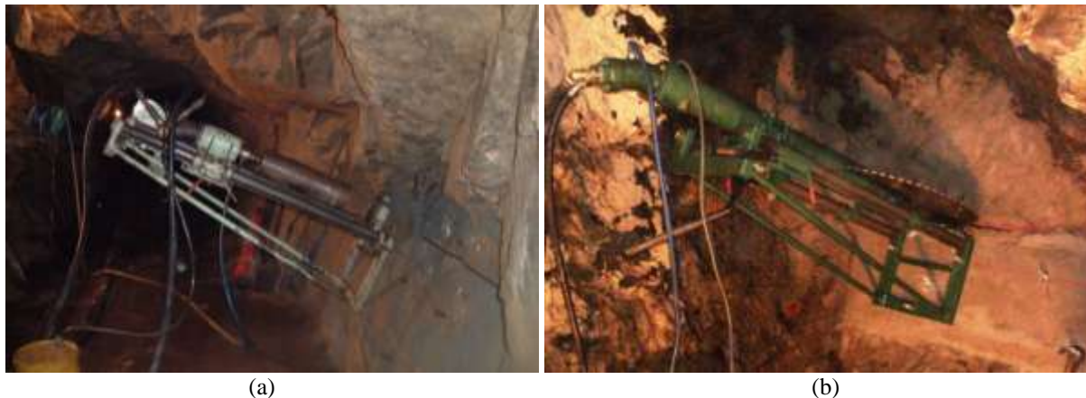
Figure 1 – Cutting machine: (a) opening the central hole; (b) cutting the slot
