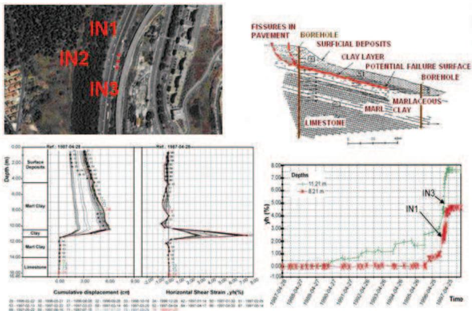
Figure 5 – Site location, cross section, inclinometer data (IN3), inferred  $\gamma_h$  data and evolution of  $\gamma_h$  for IN1 and IN3.
