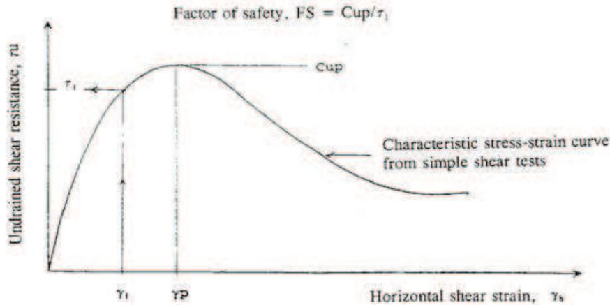
Figure 3 - Estimation of factor of safety from the estimated horizontal shear strain based on simple shear test data and inclinometer reading data (1)
