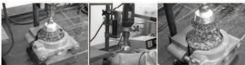
Figure 2. Brushing test of bituminous specimens
