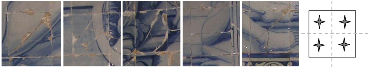
Figure 18: Fracture profiles in single tiles at the first location, and point arrangement for acquisition.
