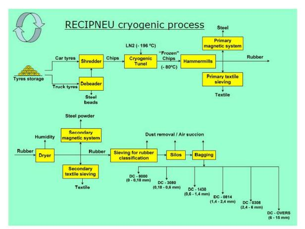
The characteristics of the crumb rubber obtained by each one of the presented processes are naturally different: cryogenic rubber particles present a "round to moderately angular morphology" (smooth faces, very small pore density and glossy appearance, similar to a "closed"/ encapsulated particle) while mechanical rubber particles generally have a very irregular surface shape, rough in texture, with high pore density (Recipneu, 2009).
