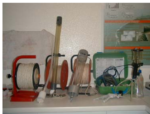
Figure 12 - Sampling devices used to collect groundwater samples
