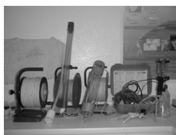
Fig. 3 – Sampling devices used to collect groundwater samples
