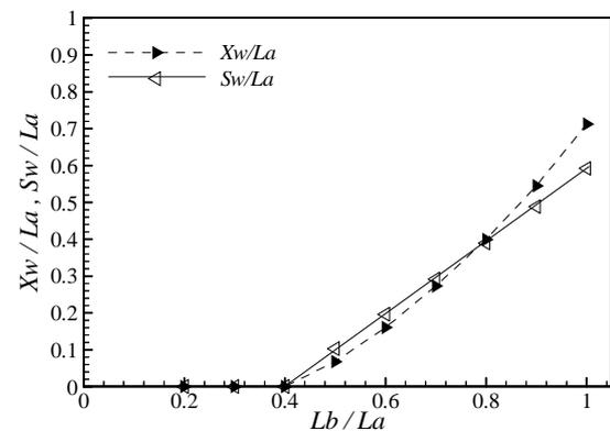
**Figure 7. Effect of AR on the vortex centre positions at  $Re=20$**
