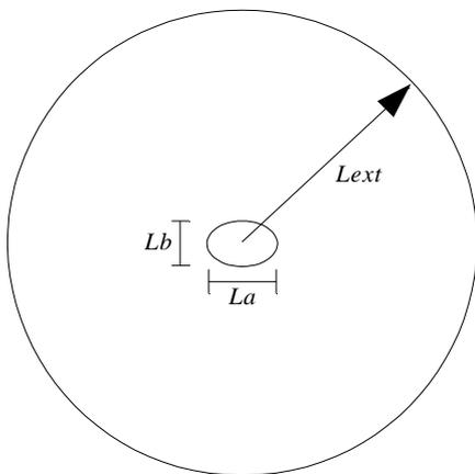
**Figure 1. Schematic of the computational domain, cylinder and outer circular boundary**
