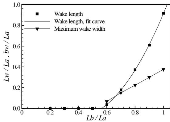
**Figure 4. Effect of AR on the wake length and width at  $Re=20$**
