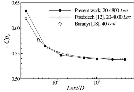
**Figure 3. Base pressure coefficient versus the computational domain extension at  $Re=20$**
