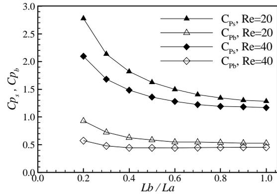
Figure 10.  $C_p$  at front stagnation point and  $C_{pb}$  versus  $AR$ , at  $Re=20$  and  $40$
