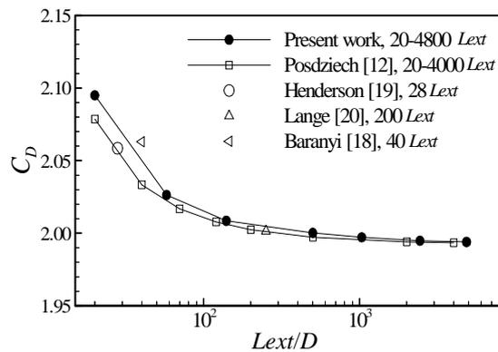
**Figure 2. Drag coefficient versus the computational domain extension at  $Re=20$**
