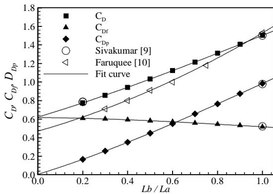
Figure 9. Drag coefficient,  $C_D$ ,  $C_{Df}$  and  $C_{Dp}$  versus  $AR$  at  $Re=40$
