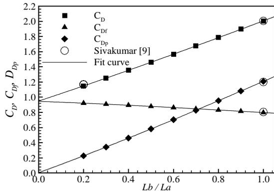
Figure 8. Drag coefficient,  $C_D$ ,  $C_{Df}$  and  $C_{Dp}$  versus  $AR$  at  $Re=20$
