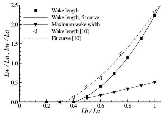
**Figure 5. Effect of AR on the wake length and width at  $Re=40$**
