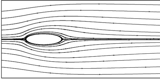
Figure 12. Flow topology at  $Re=40$  at  $AR=0.3$
