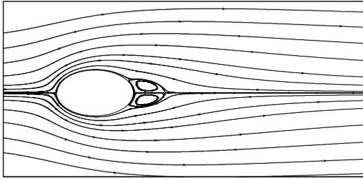
Figure 13. Flow topology at  $Re=40$  at  $AR=0.6$
