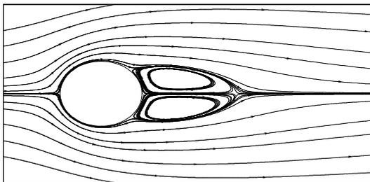
Figure 14. Flow topology at  $Re=40$  at  $AR=0.8$
