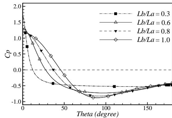
Figure 11. Effect of  $AR$  on the  $C_p$  on the elliptical cylinder, at  $Re=40$
