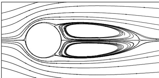
Figure 15. Flow topology at  $Re=40$  at  $AR=1.0$
