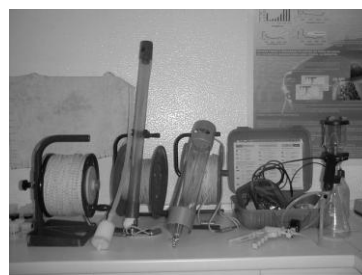
Fig. 3 – Sampling devices used to collect groundwater samples
