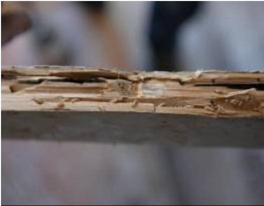
Fig. 8: Detail of the degraded wood with C. brevis attack
