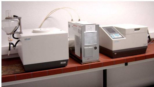
Figure 5 – Experimental apparatus related to the heat of combustion determination test at LNEC (from left to right: water supply equipment, refrigerator and calorimeter).
