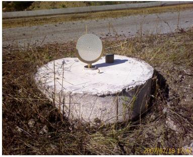
Fig. 3 Retro reflector targets on forced centering materializing an object point.
