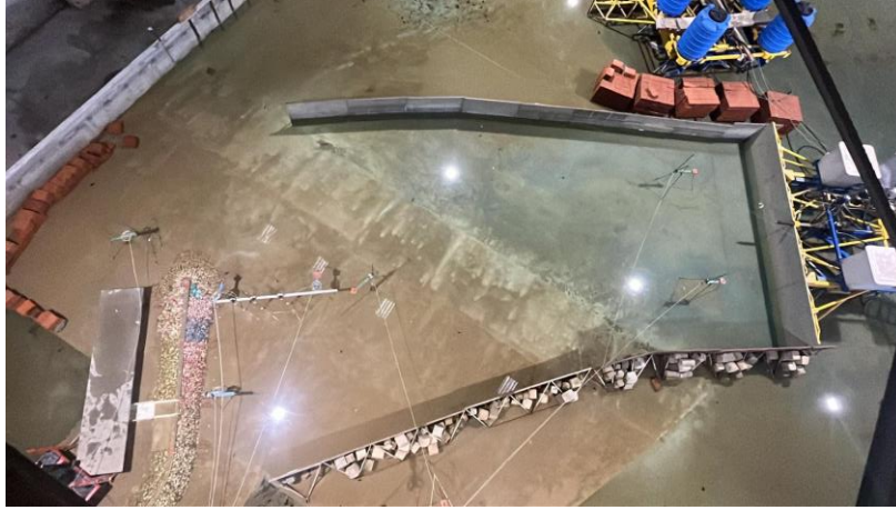
Fig. 3. Physical model of Ericeira breakwater. Scale 1:65
