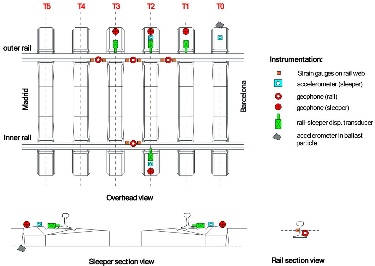
Fig. 3. Instrumentation layout in the monitored section.
