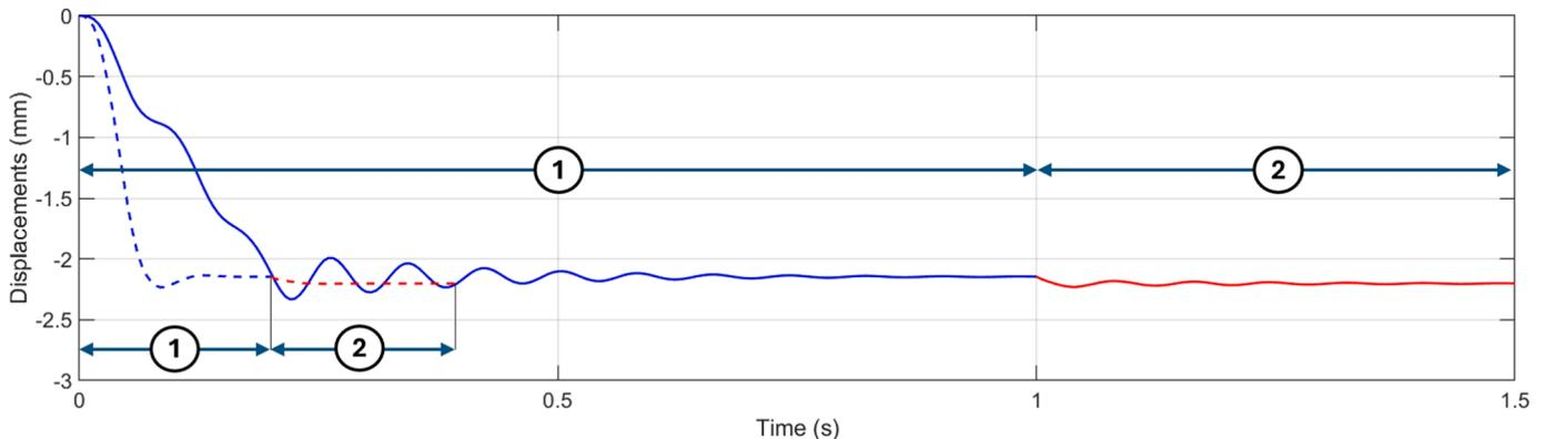
**Fig. 19.** Simulation time required to calculate the static stress/displacement field using a dynamic solution method, considering both the original damping matrix (solid line) and the augmented damping matrix (dashed line).
