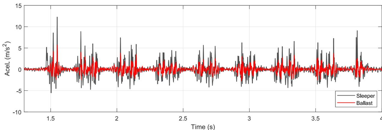
Fig. 15. Time-history of measured sleeper and ballast accelerations in vertical direction.
