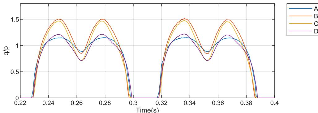
Fig. 29. Time history of  $(q/p)_{cyc}$  ratio at four locations within the ballast layer (A, B, C and D).
