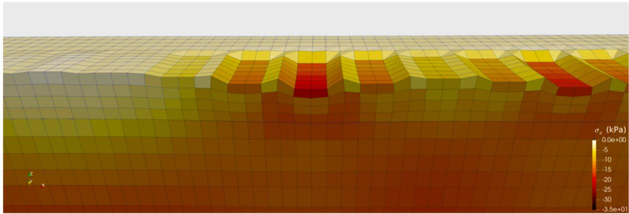
Fig. 30. Longitudinal cross-section under the rail showing the track bed layers FEM mesh deformed by instant nodal displacements (amplified 1000x) and the colors relative to the longitudinal stress  $\sigma_x$ .
