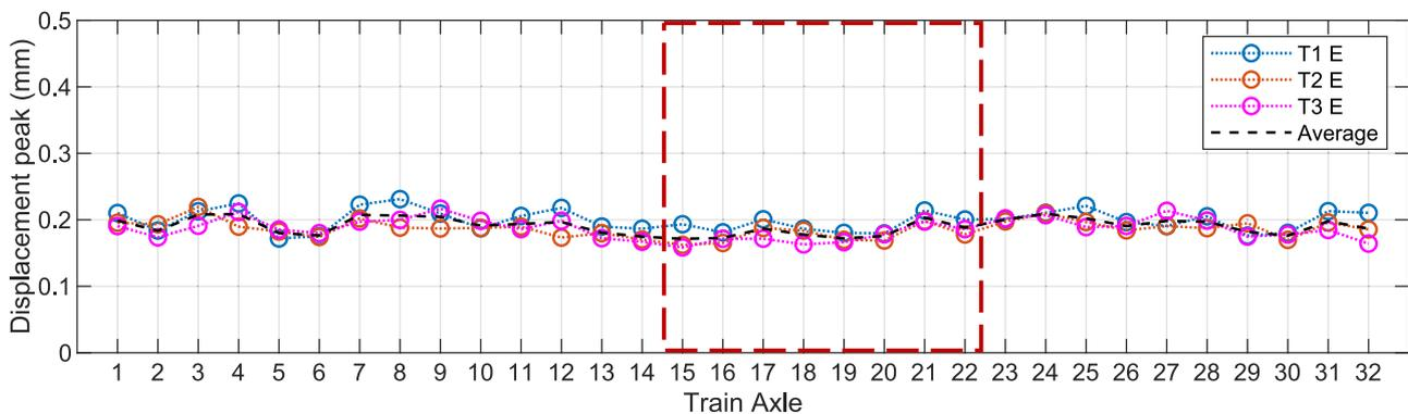
Fig. 12. Measured downward sleeper displacement peaks in the three instrumented positions of the outer alignment.
