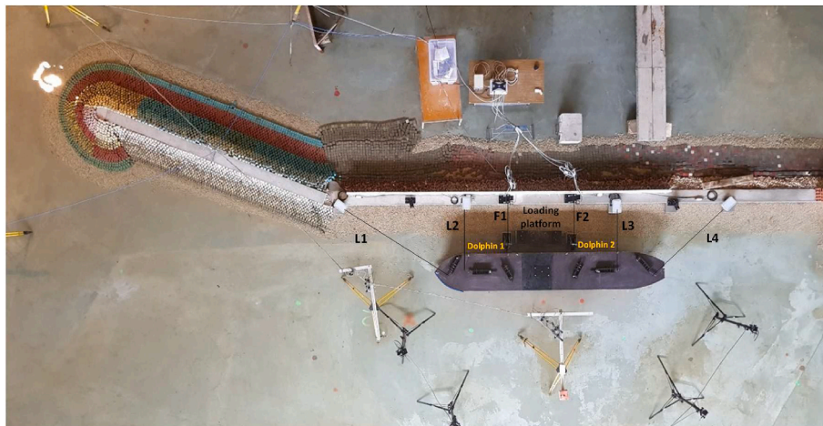
Fig. 6. The mooring arrangement in the physical model.
