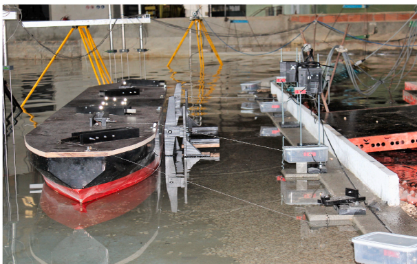
Fig. 7. Physical model of fenders and mooring lines.
