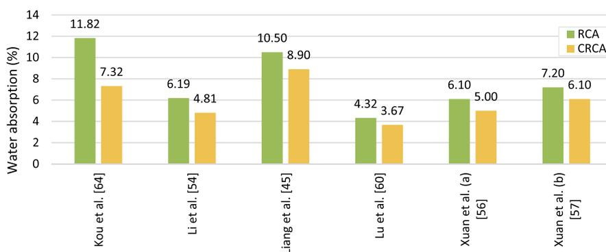
Fig. 5. Water absorption of recycled coarse aggregates before (RCA) and after (CRCA) being exposed to CO<sub>2</sub> curing.
