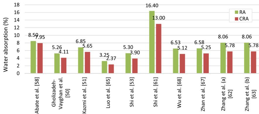
Fig. 3. Water absorption of recycled aggregates before (RA) and after (CRA) being subjected to forced carbonation.
