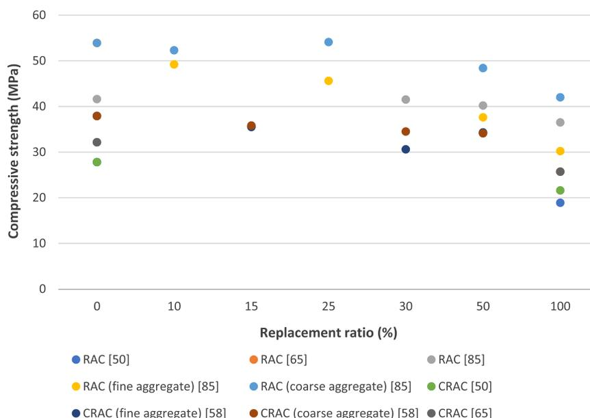
Fig. 6. 28-day compressive strength of concrete containing recycled aggregates (RAC) and carbonated recycled aggregates (CRAC).
