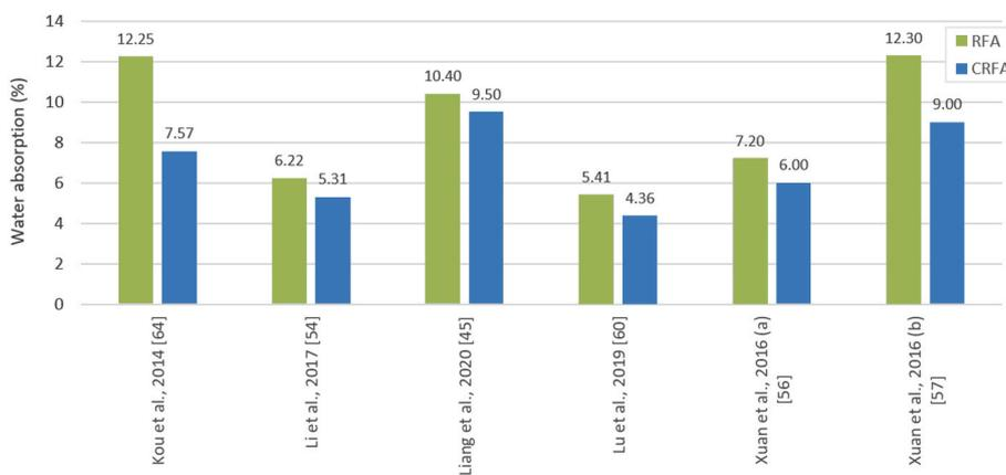
Fig. 4. Water absorption of recycled fine aggregates before (RFA) and after (CRFA) being exposed to CO<sub>2</sub> curing.
