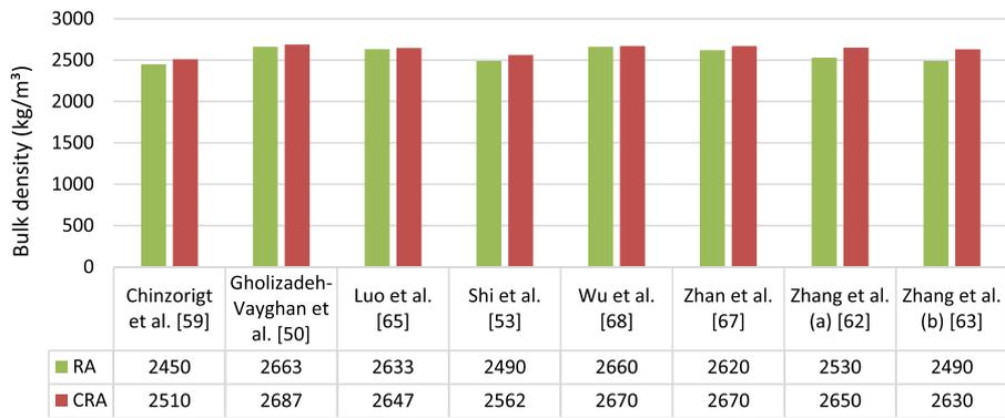
Fig. 1. Bulk density of recycled aggregates before (RA) and after being exposed to CO<sub>2</sub> curing (CRA).
