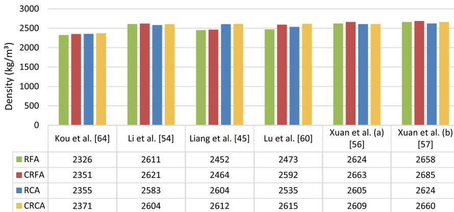
Fig. 2. Bulk density of recycled fine aggregates (RFA) and recycled coarse aggregates (RCA) before and after subjected to forced carbonation (CRFA and CRCA).
