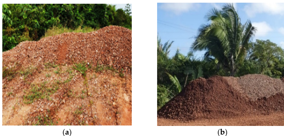
Figure 1. Photos of piles of fouled ballast in EFC Carajás. (a) Pile 1, reference code: RFBW 1; (b) pile 2, reference code: RFBW 2.
