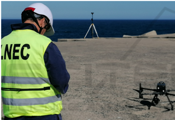
Figure 9: Preparing the flight on Sines west breakwater. Shown on top is the RTK GNSS antenna base.
