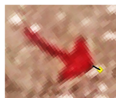
Figure 16: Point coordinated (in yellow), its image in the orthomosaic and vector between both (its length is the planimetric distance used).
