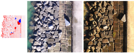
Figure 20: Displacements of blocks.
