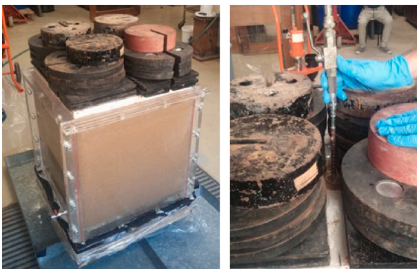
Fig. 6. Compaction load configuration (left); injection rod at the central position (right).
