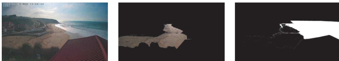
Figure 1: Left: original image; center: sand detection in HSV and masking; right: image binarization.
