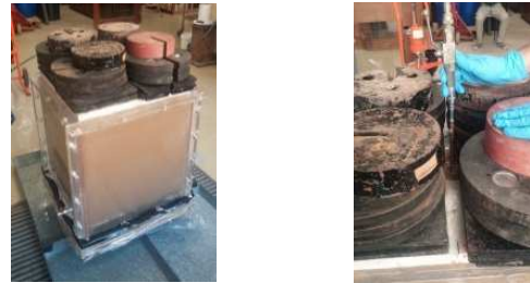
Figure 4. Load configuration (left); injection rod in the central position of the box (right).
