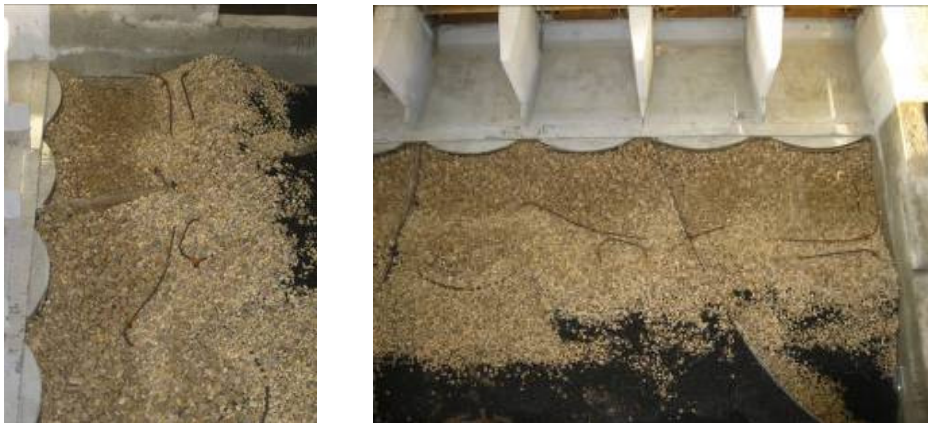
Figure 9. Riprap erosion reproduced in model assuming a revised downstream rating curve.
