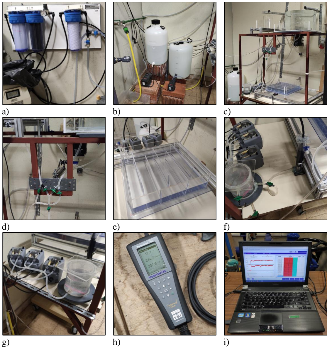
Figure A.1 – Experimental facility designed for developing tracer tests in small-scale storage tanks and determining the water residence time distribution. Tracer tests facility pictures: a) deionized water system; b) tracer solution and deionized auxiliary tanks; c) tracer solution and deionized feeder tanks (above) and small-scale tank (below); d) control valves; e) small-scale tank; (f,g) conductivity probe, hydropneumatic vessel and peristaltic pumps; h) conductivity datalogger; i) controlling software.
