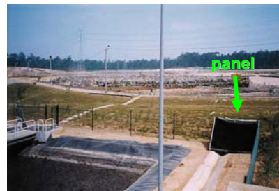
Figure 1 Example of a panel with a geomembrane sample exposed to weathering (waste landfill 3)
