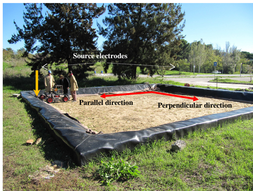
Figure 6. Electrical potential measurements with the prototype
