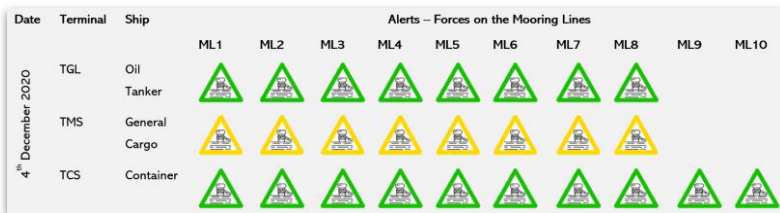
Figure 7. Dashboard of the alerts for the forces on the ships’ mooring lines.
