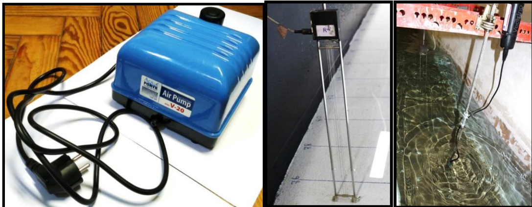
Fig. 2. Experimental equipment: Air pump (left); Resistive gauge (centre); ADV (right).
