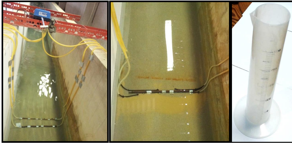
Fig. 5. Left: Air pump and tube configuration for ‘A’ and ‘B’; Centre: tube configuration for ‘C’; Right: volumetric graduated cylinder.
