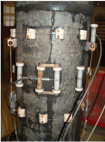
Fig. 5. Triaxial specimen with three local displacement potentiometers.
