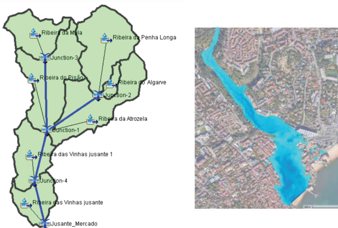
Figure 3. a) sub-basin distribution for the hydrologic modelling; b) sample inundation results of the hydraulic modelling of the 100 year return period flood.
