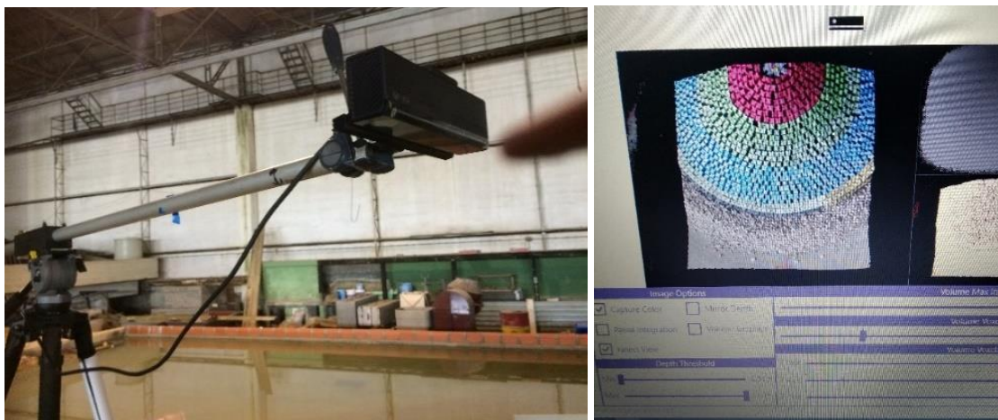
Figura 2. Sensor Kinect e interface Kinect Fusion
