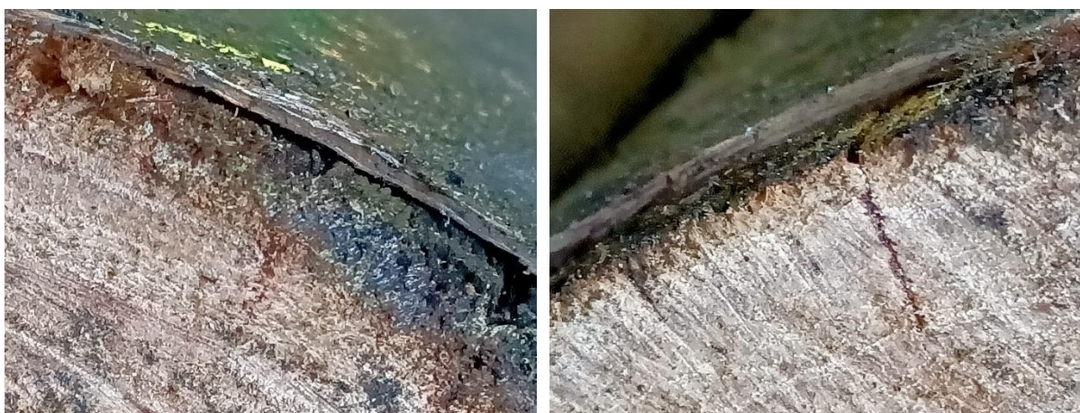
Figure 3.15 – Superficial degradation after testing (left – at 10cm of the bottom; right – at 30cm of the bottom)
