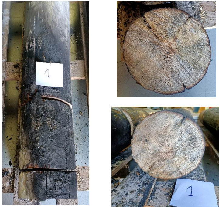
Figure 3.8 – Bottom end of pole 1 – Solution paint intumescent A & untreated pole (left – bottom end of the pole; right up – Cross-section at 10cm of the end; right bottom – Cross-section at 30 cm of the end)
