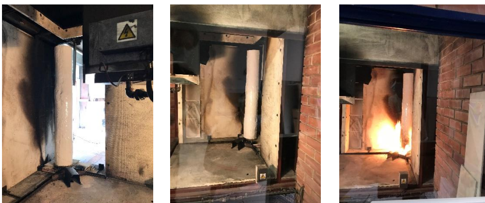
Figure 2.3 – Pole placement in the test chamber and under testing
