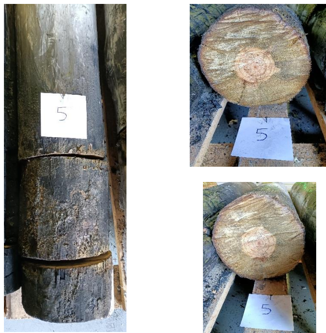
Figure 3.9 – Bottom end of pole 5 – Solution paint intumescent A & treated pole (left – bottom end of the pole; right up – Cross-section at 10cm of the end; right bottom – Cross-section at 30 cm of the end)
