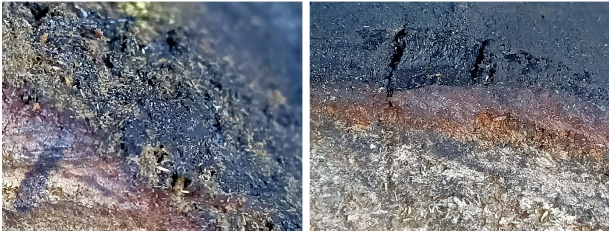
Figure 3.12 – Superficial degradation after testing (left – intumescent paint A; right – intumescent paint B)
