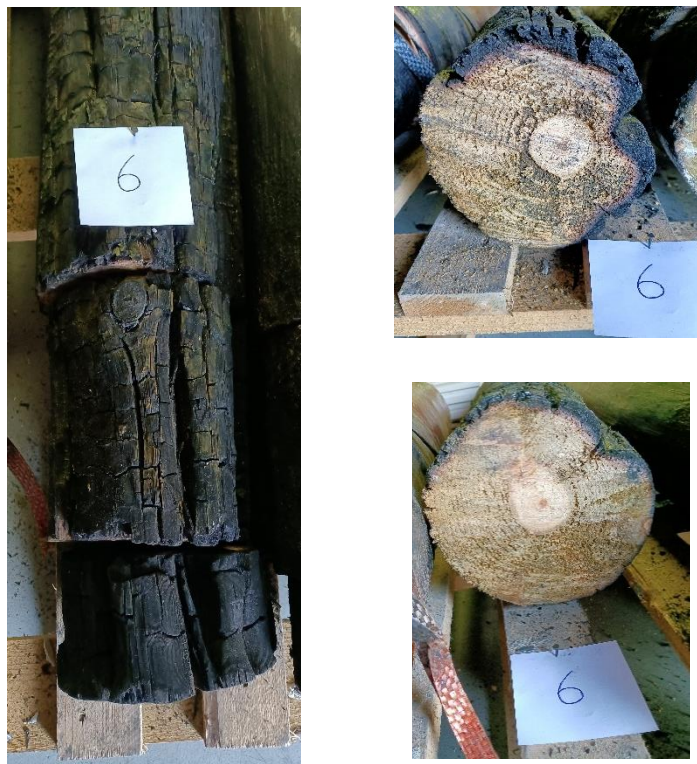
Figure 3.7 – Bottom end of pole 6 – unprotected & treated pole (left – bottom end of the pole; right up – Cross-section at 10cm of the end; right bottom – Cross-section at 30 cm of the end)
