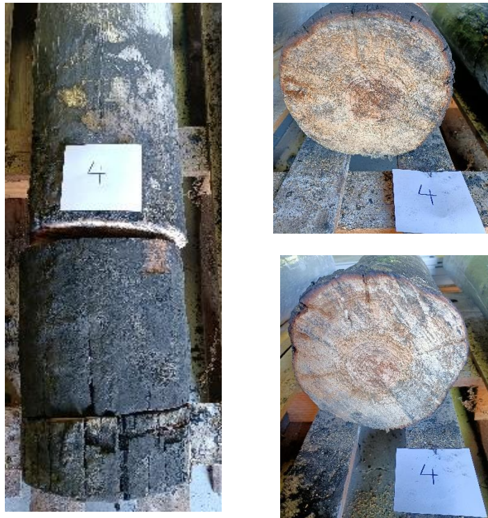
Figure 3.10 – Bottom end of pole 4 – Solution paint intumescent B & untreated pole (left – bottom end of the pole; right up – Cross-section at 10cm of the end; right bottom – Cross-section at 30 cm of the end)
