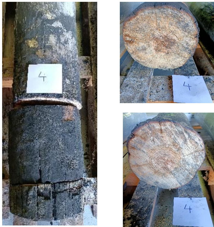
Figure 3.11 – Bottom end of pole 7 – Solution paint intumescent B & treated pole (left – bottom end of the pole; right up – Cross-section at 10cm of the end; right bottom – Cross-section at 30 cm of the end)
