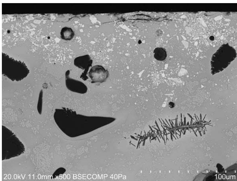
Figure 10. The presence of thin scales of a K-rich mineral in the glaze, possibly a mica, originates crystalline outgrowths with a very characteristic centipede-like morphology (seen here in Az013/04)
