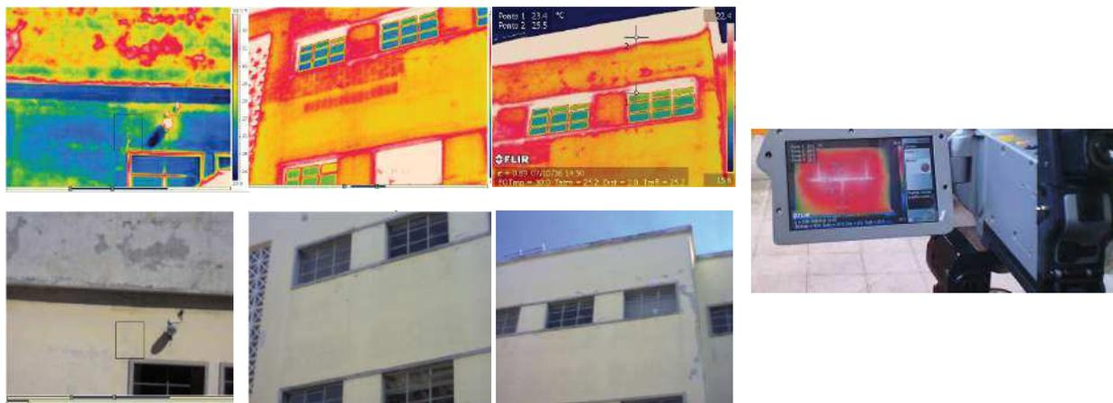
a) Facade showing rendering crack that can probably be associated, in part, to temperature variations
