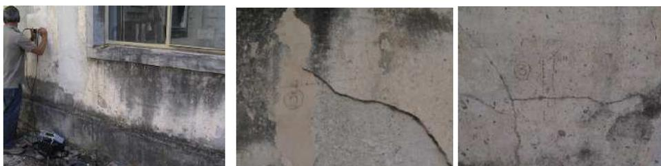
Figure 2 - Use of ultrasound testing (indirect measurements) for the detection and evaluation of anomalies occurring in a building façade [6]
