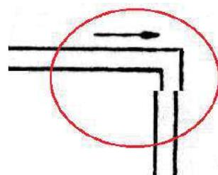
Figure 7. Example of horizontal shear cracking/oblique cracking in top of the building (roof level), due to the effect of temperature variations (movement perpendicular to the plane of the facade wall)
