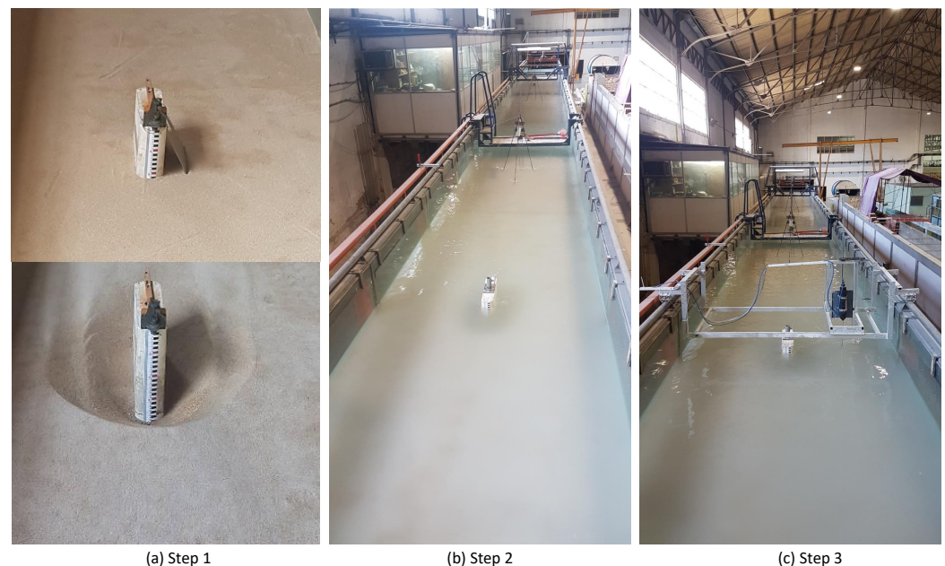
Figure 4. Setup for the flow velocity measurements.
